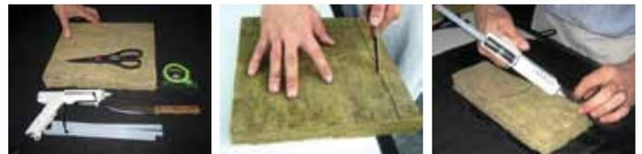
Easily cut with a serrated or craft knife for quick and simple installation.
